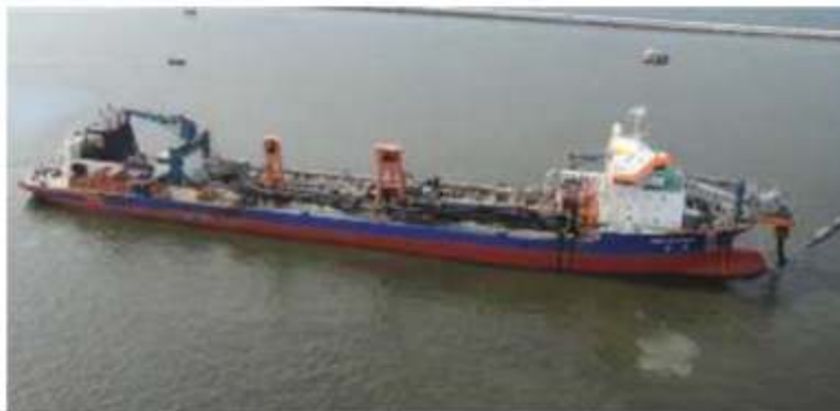
Gambar 5 Trailing Suction Hopper Dredger 30,000 m 3
